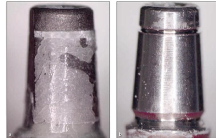
**Fig 7** (a) Cohesive and (b) adhesive failure between abutment and cement.
